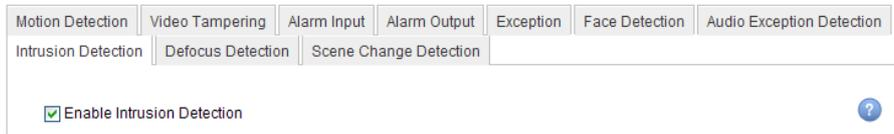
Figure 6-13 Setting Intrusion Detection on IP Camera
