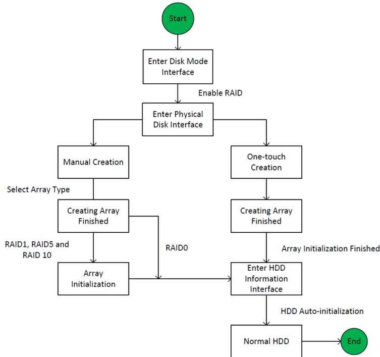
Figure 13-1 RAID Working Flow
