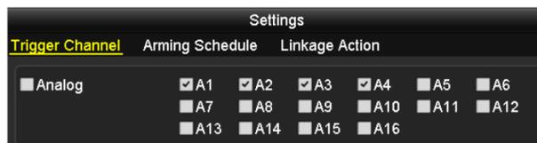
Figure 8-3 Set Trigger Camera of Motion Detection
