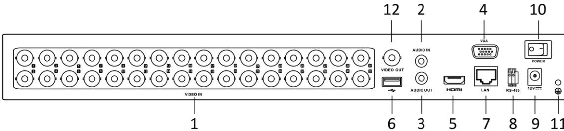
Figure 1-14 Rear Panel of DS-7200HQHI-K (with 32 Video Inputs)
