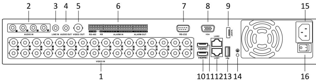
Figure 1-20 Rear Panel of DS-7300HUHI-K4 (with 32-ch Video Inputs)
