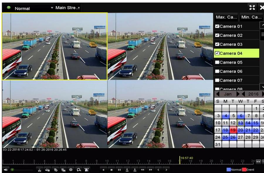
Figure 6-26 4-ch Synchronous Playback Interface
