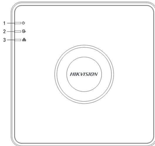
Figure 1-1 Front Panel of DS-7100HQHI-K1
