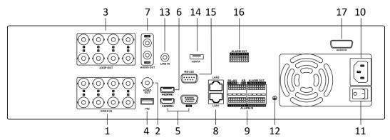
Figure 1-18 Rear Panel of DS-9000HUHI-K8 (with 8 Video Inputs)
