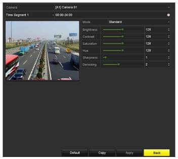
Figure 15-5 Image Settings Interface (Analog Camera)
