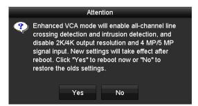
Figure 17-6 Enable Enhanced VCA Mode
