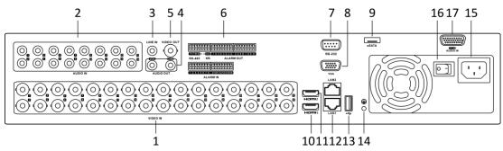
Figure 1-21 Rear Panel of DS-8100HQHI/HUHI-K8 (with 32-ch Video Inputs)
