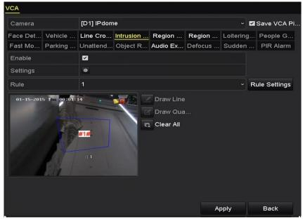
Figure 10-9 Draw Area for Intrusion Detection
